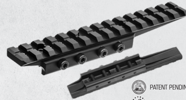
MNT-DTW145 Universal Dovetail To Picatinny Rail Adaptor • Precision Machined from Aircraft Aluminum with a Matte Black Finish • Compatible with 9mm-11mm Dovetail Rails
